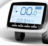
Display with speedometer, distance meter, and battery capacity
